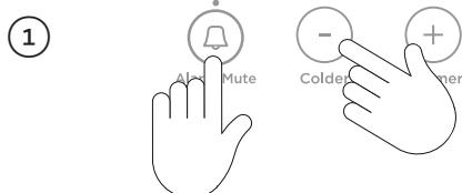
Press and hold **Alarm**, **Mute** and **+** together for 4 seconds then close the door(s). The ice tray will flip twice and empty the water into the bin below. The ice tray will flip only after the doors are closed.
