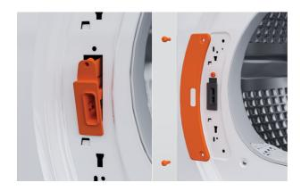
**5.** Rotate latch and insert on opposite side of dryer. Secure with screw.
