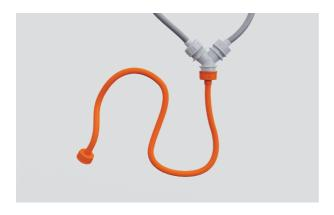
**8.** Connect the straight hose to the bottom of the Y joint. The other end of the straight hose will connect to the cold tap.
