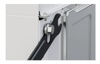
**5.** Using the spanner provided as a spacer, ensure a 4mm gap is left between the bolt head and the chassis.
