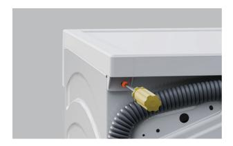
1. Remove screws from washer using a screw driver or drill on the lowest torque setting.
