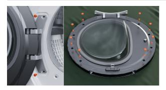
1. Unscrew hinge screw using a T25 torx screwdriver then remove door and place face down on a protected surface. Remove plugs (x8) from inner door flanges, then remove screws.
