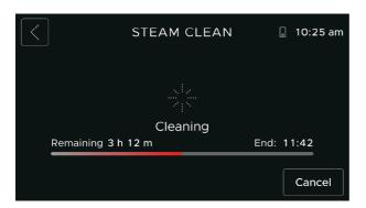
2. Remove all shelves and accessories and fill the water tank, then start the cycle. A progress bar will show while STEAM CLEAN is running, and while a cooling cycle is running.
