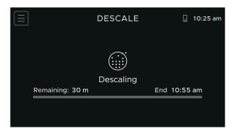
2. Remove the tank and fill it with descaling solution, then reinsert the tank to start the cycle.
