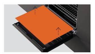
2. Lift the pane up to remove it, and place it on a flat, protected surface. Clean the glass as required. See 'Care and cleaning.'
