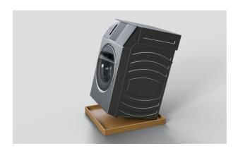
2. Remove any packaging and accessories from the top of the machine. Lift the washer off the base and remove any packaging and accessories from the base.
