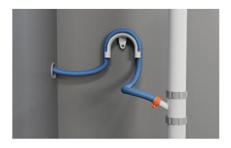
**6.** B) **Spigot installations:** Drill out blanking insert from the spigot.
