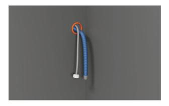
**4.** Route the power cable and hoses through service holes. Ensure power will remain accessible following install to allow access for any future product maintenance.
