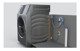
1. Carefully move the appliance into place without damaging the rubber levelling legs, as this can cause increased vibration. Spraying window cleaner on the floor may help it slide more easily or use specialist equipment if available to installer.
