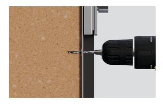
1. Using the product as a guide, pre-drill  $2 \times 3$ mm pilot holes.
