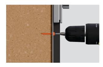
**2.** Secure oven to cavity using the 2 x screws provided.
