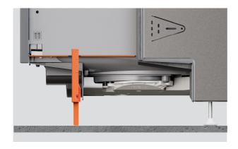
1. Open the bottom drawer. Rotate the toe kick so the tabs are resting on the floor.
