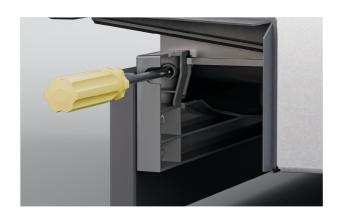
**5.** Slide mounting bracket along T rails until it is in position.
