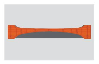
For a toe kick depth of 40mm to 88mm, the shallow curve (profile A) will be cut from the toe kick.
