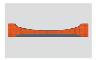
For a toe kick depth of 88mm to 100mm, the wider curve (profile B) will be cut from the toe kick.
