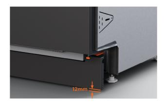
**4.** Snap off the top tabs. Slide the pre-finished toe kick along the T rails into position. Ensure there is a 12mm gap between the toe kick and the floor.
