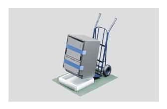
**3.** To detach the base, use a trolley to lift the dishwasher from the rear, then pull the base off.
