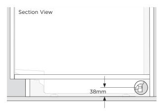
2. The center of the hole should be a maximum of 38mm from the floor or the bottom of dishwasher feet.
