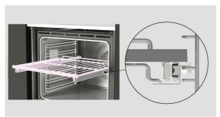
2. To refit, place the shelf on top of the side racks, and push into the oven, with the guard rail at the back.
