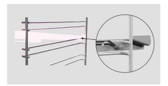
**3.** Ensure the rear tags are hooked over the side racks on both sides.
