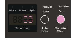
Press **OPTIMISE WASH** until [1] is displayed on the screen. Your washer will now adjust the cold temperature to approximately 20°C.
