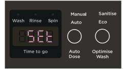
Press and hold the desired wash modifier for 3 seconds. A long tone will sound and 5EE will display onscreen.
