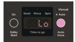
Ensure Auto Dose is set to AUTO. Liquid detergent will be dosed automatically. Do not add detergent to the manual dispenser when using AUTO.
