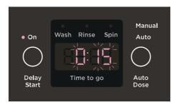
Press **DELAY START** to cycle through the delay times. Press **▶II** to start the countdown. When **DELAY START** has begun, the time will begin counting down.
