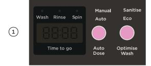
With the display panel turned off, press and hold AUTO DOSE and OPTIMISE WASH for 3 seconds.
