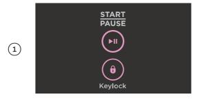
With the washer on at the wall, but off at the display, press and hold **6** and ►II together for 3 seconds.
