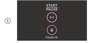
With the washer on at the wall, but off at the display, press and hold **6** and **>11** together for 3 seconds. **aPAd** will show on the display.
