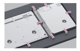
1. Fit the securing brackets to the base of the product. For benchtops thinner than 25mm, use the longer clamp screws.
