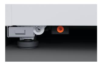
2. Adjust the front of the product by turning the outer screws clockwise to lower the feet until the product is off the wheels.
