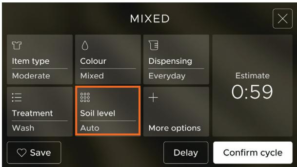
5. Press **SOIL LEVEL** to select a soil level option, or use **AUTO**. **AUTO** senses the soil level and adjusts the wash time and detergent dose to suit.
