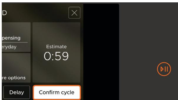
5. Press **CONFIRM CYCLE**, then press the **START/PAUSE** button to start the wash cycle.
