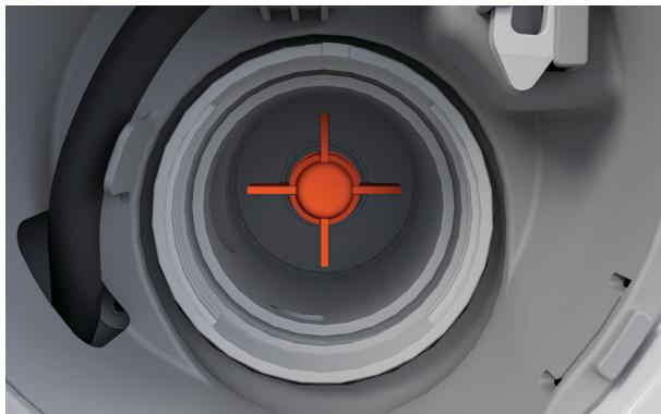
**4.** Check and clear the cavity behind the filter, and check that the impeller behind the filter moves freely.
