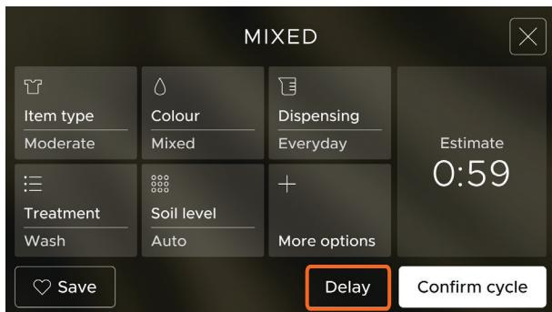
1. After setting the cycle, press **DELAY** to open the Delay screen.
