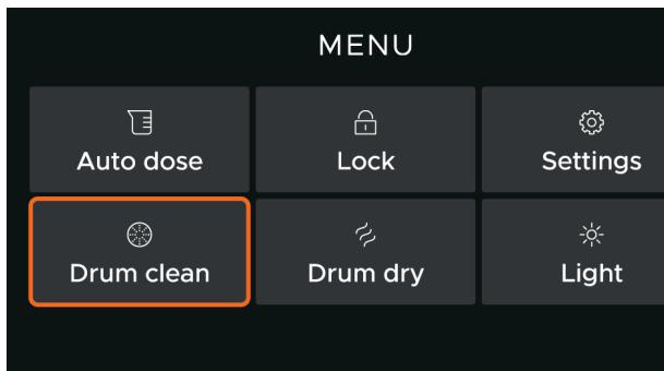
2. Go to **MENU** and select **DRUM CLEAN**. Press **CONFIRM**, then press the **START/PAUSE** button to begin the cycle.
