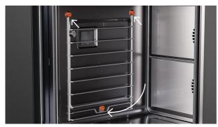
**3.** To replace, fit the top of the rack into the studs, then push the base of the rack flush against the side of the oven. Refit the nut at the base of the rack, and tighten it to secure.
