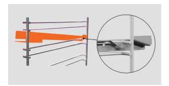
**3.** Ensure the rear tags are hooked over the side racks on both sides.
