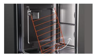
2. Pull the base of the rack clear of the screw, then pull the rack down to separate it from the studs at the top.
