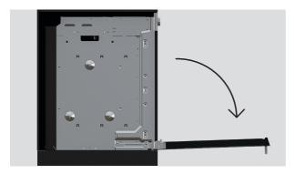
1. Open the door fully, and locate the hinge locks on either side of the door.
