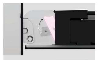
2. Locate the hinge locks on either side of the door. Push the locks upwards to release.
