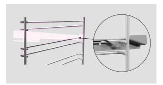
Ensure the rear tags are hooked over the side racks on both sides.
