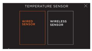
1. Select a function or method then press OPTIONS. Select TEMPERATURE SENSOR, then WIRED SENSOR.
