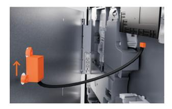
**2.** Check that the module is oriented correctly to ensure proper function.
