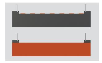
**5.** For a toe kick depth of 40 - 100mm, align the custom panel along the lower edge of the toe kick mount.
