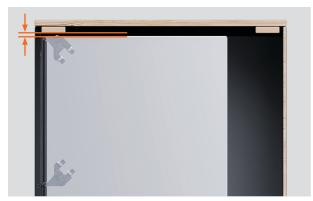
**3.** Adjust the dishwasher height to 3 to 5mm below the cavity height.
