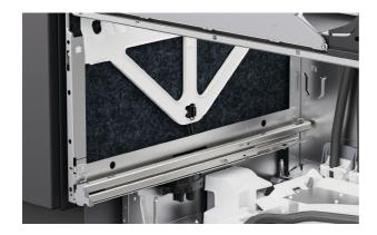
**5.** Refit insulation ensuring it is positioned correctly and will not obstruct the drawer runners.
