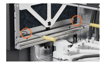
**4.** Insert screws through the two holes on each side of the chassis.
