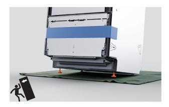
**4.** Tilt the dishwasher to rest on its back feet and unscrew or tighten the front feet.
