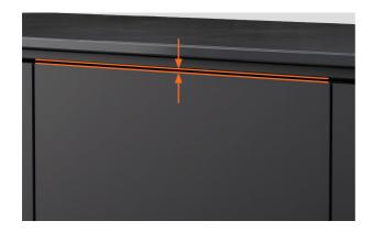
**5.** Place the top panel onto the dishwasher and check that the panel gap is minimum 2mm. Remove the panel and adjust again if necessary.
