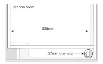
1. A minimum 57mm diameter service hole is required in the cabinet side.
