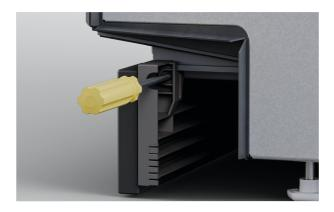
7. Slide mounting bracket and toe kick along the tub rails.
