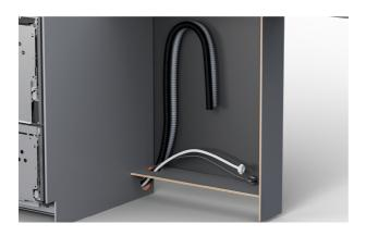
**6.** Service holes can be routed from the dishwasher cavity, into the toe kick space. Then through to the adjacent cavity.
