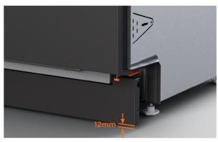
**4.** Snap off the top tabs. Slide the jig and toe kick along the T rails into position.
