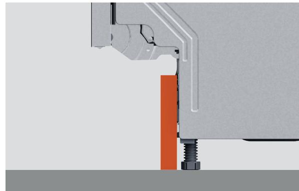
4. Firmly press the rubber side of the foam strip against the toe kick area, ensuring the foam forms a seal between the floor and the product.
