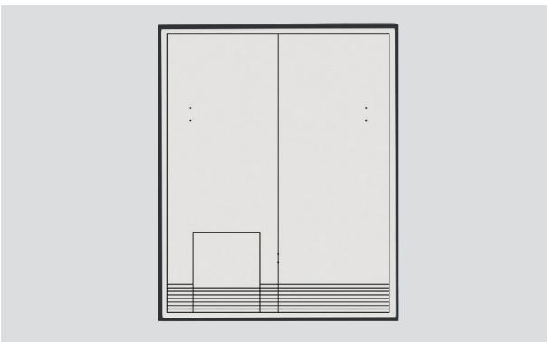
1. Using the door template as a guide, pre-drill all holes into the door panel.
