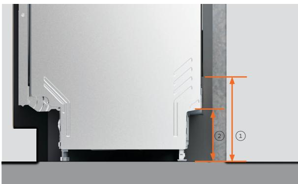
3. Measure the distance from the lower edge of the black backing to the floor ①, and the distance from the recess to the floor ②.
