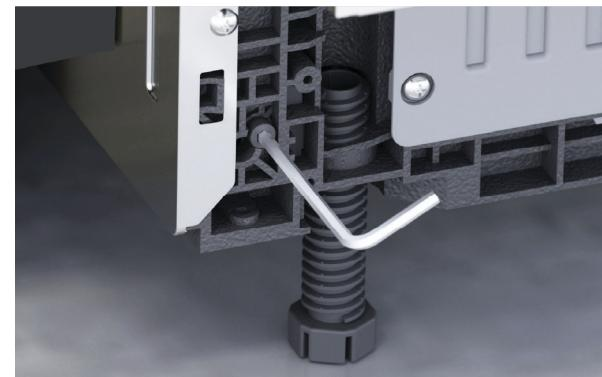
5. Use a 4mm Allen key to adjust the door tension. Rotate clockwise to increase tension, rotate counter-clockwise to decrease tension.
