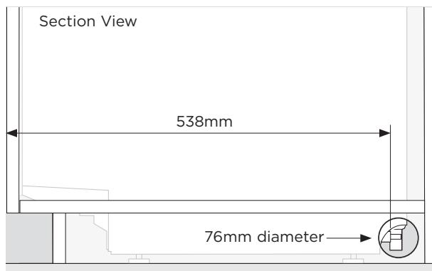
1. A minimum 76mm diameter service hole is required in the cabinet side.
