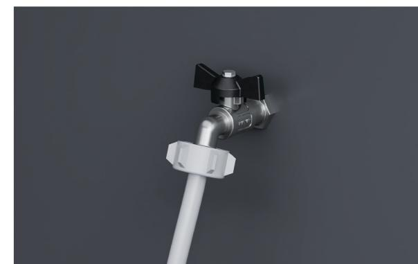
3. Hand-tighten into place. Using a spanner or pliers, turn a further 180° to secure. Avoid over-tightening.
