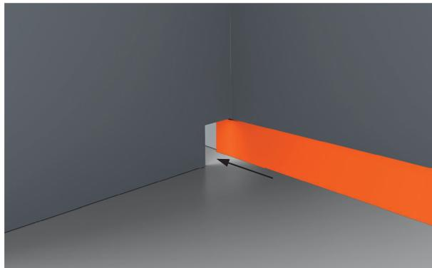
2. If possible, cut a piece of foam to line the back wall adjacent to the dishwasher.
