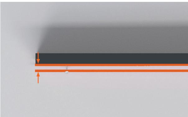
2. Fit x2 16mm screws into the pre-drilled holes. Ensure there is a minimum space of 3mm between the screw-head and the panel.
