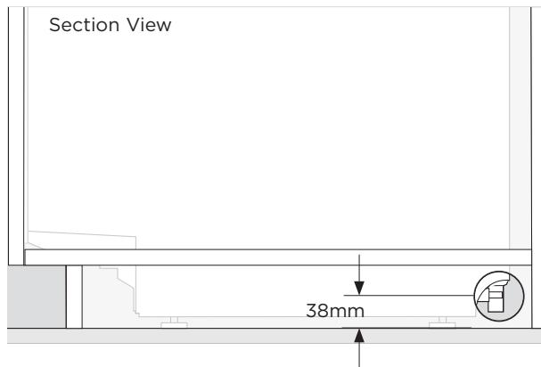
2. The centre of the hole should be a maximum of 38mm from the floor or the bottom of dishwasher feet.
