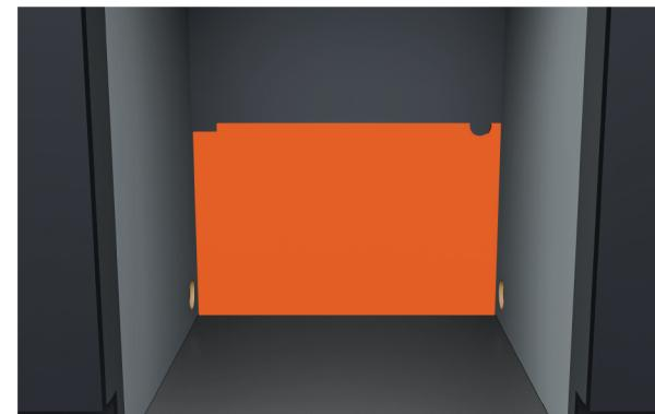
5. Peel half of the backing off at the bottom of the foam. Start at the bottom where the wall meets the floor and continue to peel the backing off as you move upwards.
