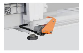
9. Roll washing machine into alcove and check alignment. To do this, use the supplied 6mm hex key, rotate clockwise to lower both sets of wheels via the adjustment screws.
