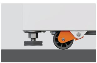
**18.** Open plinth to access wheels. Turn the adjustment screw counter-clockwise to retract the wheels. Ensure the wheels are fully raised off the floor.
