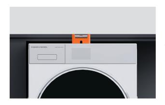
**13.** Check that products are still level. Adjust plinth feet if necessary.
