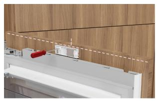
**6.** Close the door and apply pressure to secure. Open the door and fit 2x screws to the striker plate. Clip striker plate cover into place.
