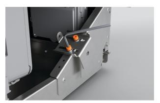
**3.** Re-tighten the cap screws.
