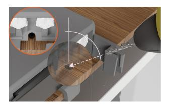
**4.** Slot the accessory onto the shoulder bolts. Pre-drill pilot hole at a 45° angle using the accessory as a guide.
