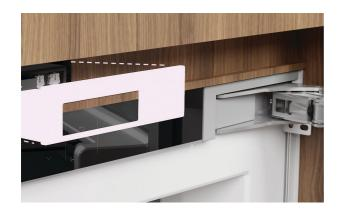
**9.** Fit the bridge trim. Place the accessory cabinetry housing and slot lens cover in place.
