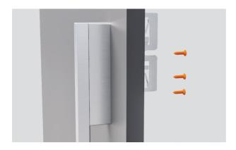
**4.** Fit the handle to the panel using four M5x25 hex screws. Ensure handle fixings do not interfere with side brackets.
