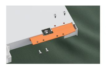
**3.** Install the new upper adapter bracket into the other side of the top of the door with four M5x10 screws.
