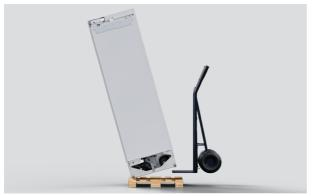
**3.** Tilt the appliance forward slightly and insert the hand truck between the pallet and product.
