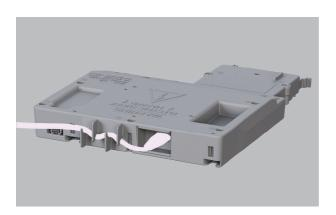
2. Route the accessory power cord from rear of the product through to the front corner. Connect the power cord to the accessory before threading through strain relief bracket.
