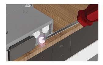
**8.** Fit the front screw through the pilot hole using a Phillips screwdriver. Adjust settings if required.
