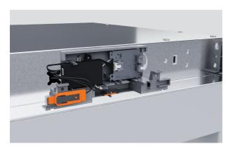
**6.** Clip the hall sensor into the sensor housing in the pocket closest to the centreline of the cabinet before pressing the interceptor board harness into the forks.
