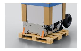
**5.** Removing the remaining brackets.
