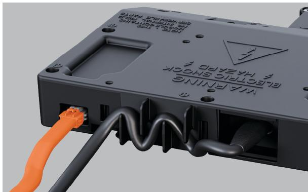
6. Plug the communication cable into the back of the unit.
