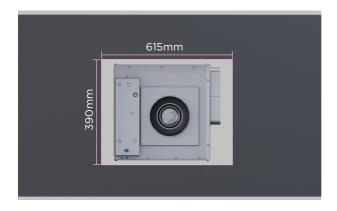
2. Create a 615x390mm cutout in the base of the cavity for the external blower.
