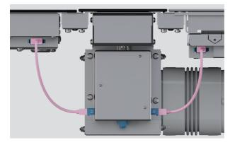
1. Link each product to the adjacent product using the supplied communication cables. Ensure 8-pin plugs are only connected to 8-pin sockets and 6-pin plugs connected to 6-pin sockets.
