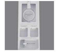
If detergent and softener is set to Auto, ensure that liquid detergent and softener has been added to the auto dose-compartment
