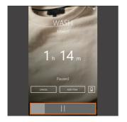
Press || to pause cycle. The washer door will stay locked if the water level is high or the temperature is too hot. It will unlock automatically once it's safe to open.
