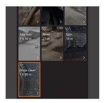
Select the **DRUM CLEAN** wash cycle under wash cycles on your machine. Follow the instructions on the screen.
