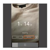
Press ADD ITEM at any time during the wash/dry phase of the cycle to add or remove an item. The door will unlock once water level has reduced or drum has cooled down, which may take a few minutes. It will unlock automatically once it's safe to open.
