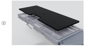
Place the foam back on the filter using the locating tabs for guidance.
