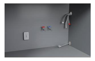
**4.** Route the power cables and hoses through service holes.
