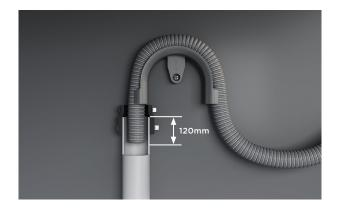
**5.** Ensure the hose does not extend more than 120mm into the standpipe to prevent wastewater siphoning back into the tub.
