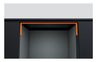
**3.** Apply tape to top edge of cabinet ensuring it is centred and set back 10mm from the front edge.
