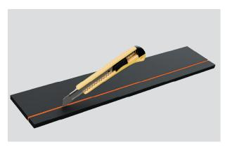
**2.** Cut off the excess foam and check it fits under the machine. Adjust if necessary.
