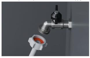
1. Check that the supplied rubber washer is inserted into the coupling.
