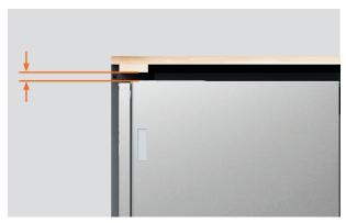
**3.** Adjust the dishwasher height to 3-5mm below the cavity height.
