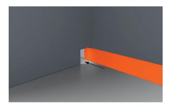
2. If possible, cut a piece of foam to line the back wall adjacent to the dishwasher. Refer to steps 3 for sticking foam to the wall.
