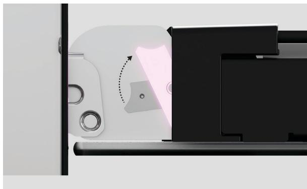
2. Locate the hinge locks on either side of the door.
