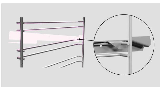
2. Ensure the rear tags are hooked over the side racks on both sides.
