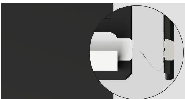
**5.** When replacing the second middle pane, ensure the metal bracket is still in place and correctly positioned at the bottom of the glass.
