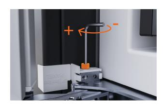
**6.** Expand the lower spacer to create an even gap between product and alcove.
