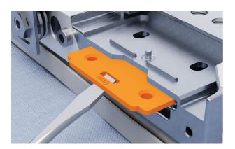
**6.** Use a flathead screwdriver to remove the inside plates. Move to the other side ensuring the rounded corners face the inside.
