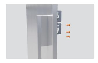
**5.** Fit the handle to the panels using four M5x25 hex screws.
