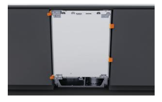
1. Push product in until the depth gauges touch the front of the alcove. Ensure power cord is not trapped.
