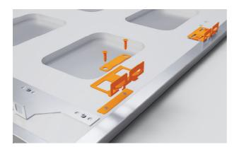
**4.** Align the side brackets to the panel. Secure using the supplied screws. Ensure brackets are fitted tightly and the fasteners are secured straight.
